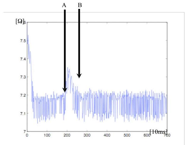
Fig. 5: Measured resistance of the actuator.
