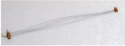
Fig. 1. The developed SMA wire bundle actuator.
