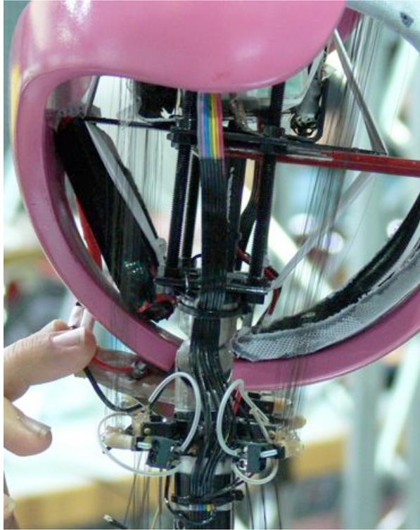
Fig. 9: Actuators integrated in the humanoid robot Lara.
