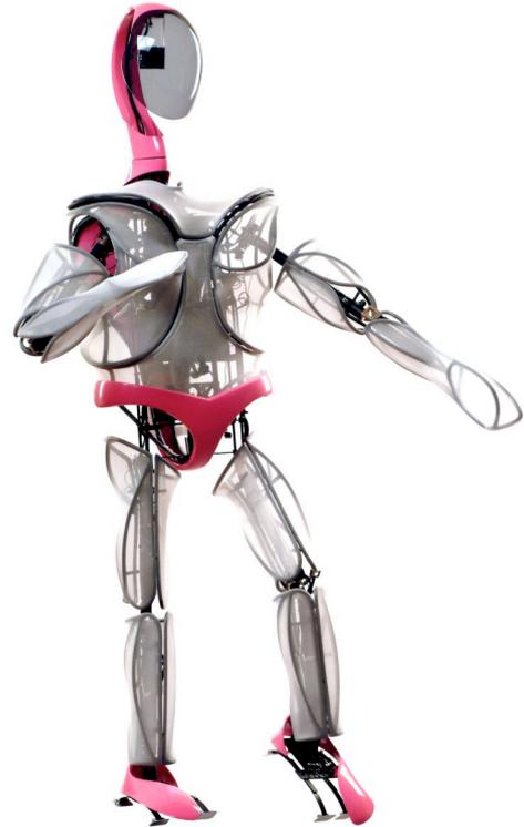
Fig. 8: Humanoid robot "Lara" actuated by 34 SMA wire bundle actuators (cf. [www.lara-robot.de](http://www.lara-robot.de)).
