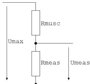
Fig. 4: Indirect measuring of actuator's current.
