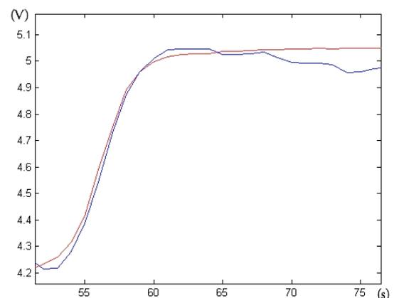
Fig. 3. Relation between resistance (4.2V ~ 8.2Ω, 5.0V ~ 7.5Ω,) and contraction (4.2V ~ 22cm, 5V ~ 20.3cm) (contraction: red line, resistance: blue line)
